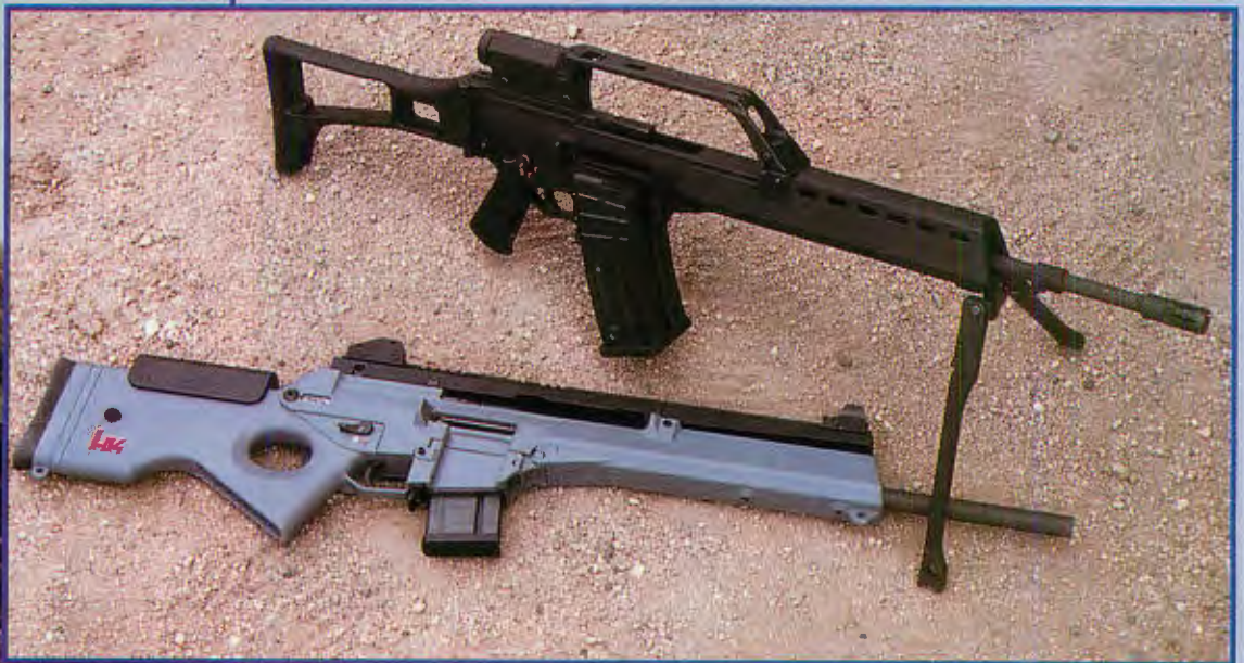
(left) Brass flies as this officer fires a burst from his G36K carbine. He is using the 1.5X optical sight. Above it is the red dot reflex sight also integral with the carrying handle. (above) The standard G36 rifle (top) is seen with the semi-automatic only SL8-1 rifle that any law-abiding citizen can own.
